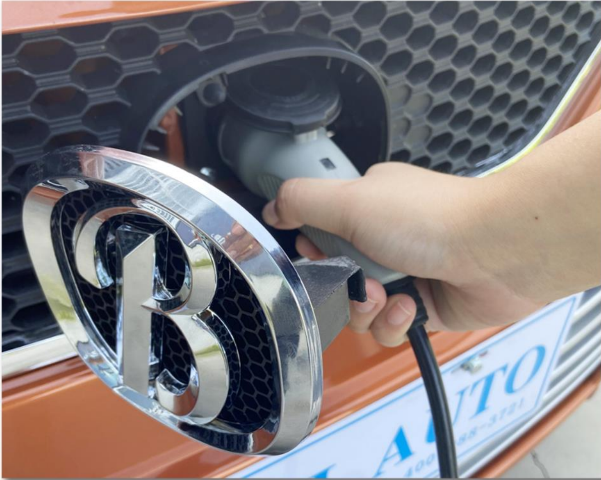
◀ CAR CHARGING PORT
